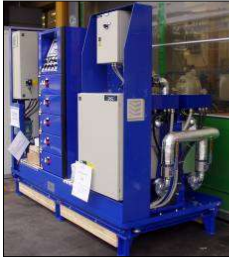
Fuel conditioning module
