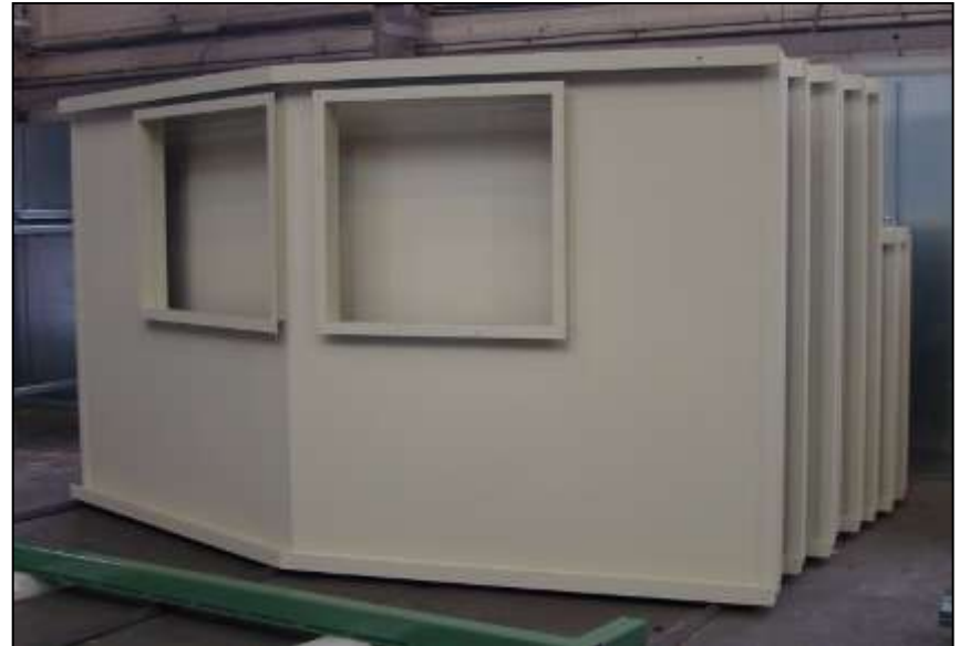
Acoustic enclosure roof panels in storage
